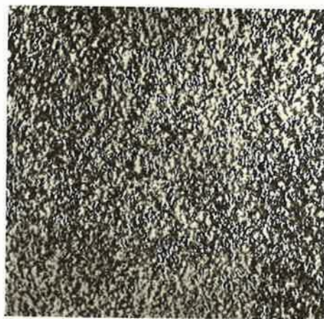
Fig 5. Bad IV i = 30 \frac{\text{mA}}{\text{cm}^2} Vergröss. 30 ×
