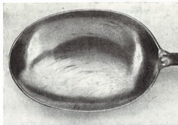
Figure 1. Concave inner surface of a spoon employed as the leading side of an exchangeable stirrer blade of a pulp impeller. The initial resin deposition takes place at this leading surface, and later shear forces force the resin to flow along the surface and leave typical flow tracks.
