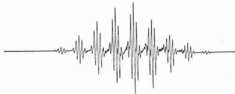
Figure 1. Electron resonance spectrum of the reaction mixture obtained when 4,4'-dimethoxybiphenyl was treated with potassium in dimethoxyethane. The spectrum of the biphenyl anion radical dominates.
