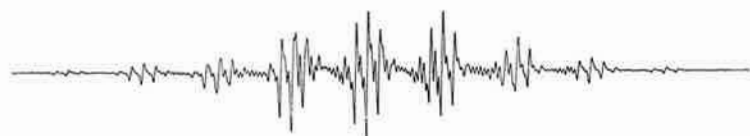
Figure 2. Electron resonance spectrum of the reaction mixture obtained when 4,4'-dimethoxybiphenyl was treated with potassium in dimethoxyethane. The spectrum was recorded immediately after the solution was placed into contact with the distilled potassium.
